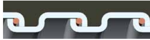
Square-Locked Design with integral bonding wire 3/8" through 1-1/4"
